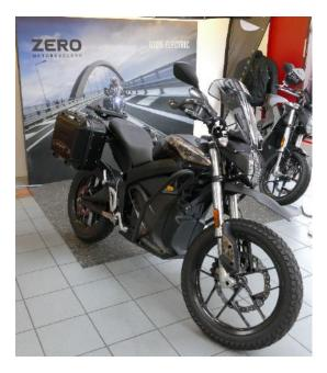
battery 14.4kWh model format, takes about 2.5 hours. A long time for a coffee break maybe but it still means you're charging half the "tank" in about an hour.
